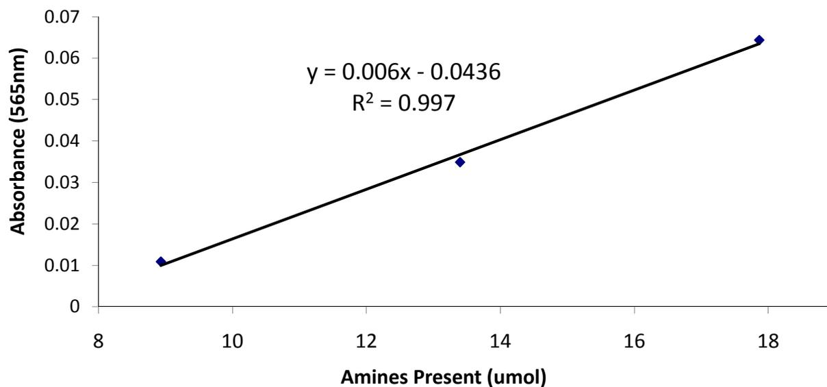
**Figure 2.2.** Typical Calibration Curve for Ninhydrin Assays. Absorbance values as a function of amine concentration for three calibration standards prepared with aliquots of a 1 mg/mL APS solution in ethanol. Calibration standards were prepared daily for all ninhydrin runs provided in Figure 2.3 and Figure 2.4, and the associated calibration curve and equation were used to quantify the amine density for the ninhydrin reactions performed with APS silica.
