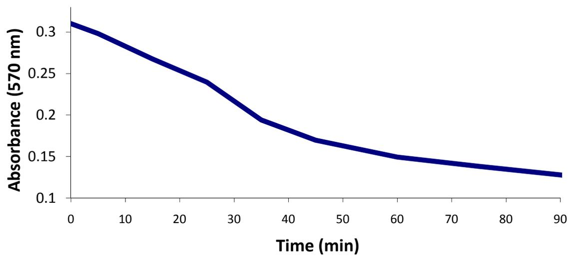
**Figure 3.5.** Micelle Monolayer Determination. The Absorbance at 570 nm of a solution containing phenol red indicator and micelles stirred with Davisil silica over time. The adsorption of indicator encapsulated micelles onto the silica resulted in the decrease of solution absorbance. The experiment was run for a sufficient time to allow for the micelles to adsorb completely, and the micelle monolayer capacity on the surface was determined based on the remaining number of micelles in solution.
