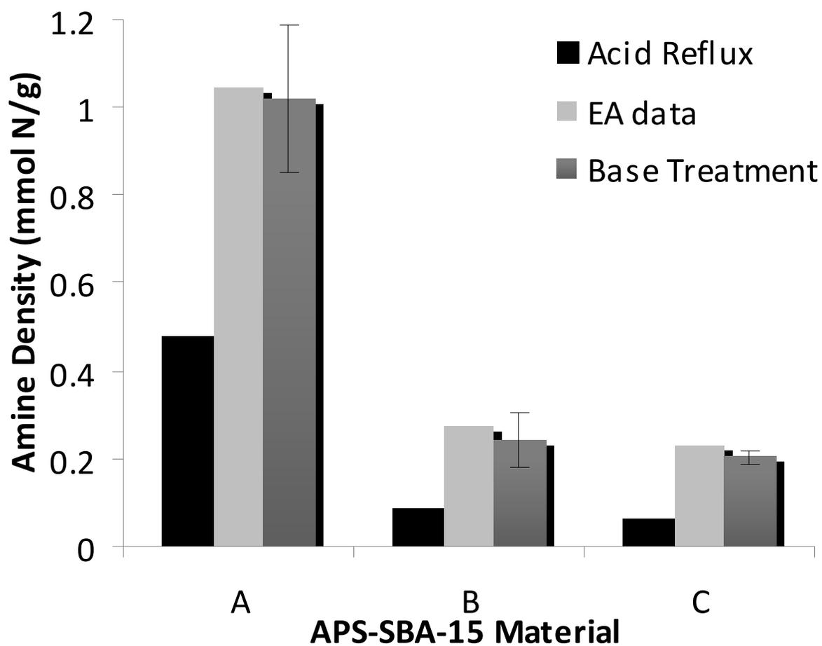
**Figure 2.4.** Ninhydrin Tests on APS-SBA-15. Tests were performed after treatment in refluxing ethanol and after an additional treatment with  $N(CH_3)_4OH$  in refluxing methanol. Ninhydrin tests are compared to the expected results determined from elemental analysis.
