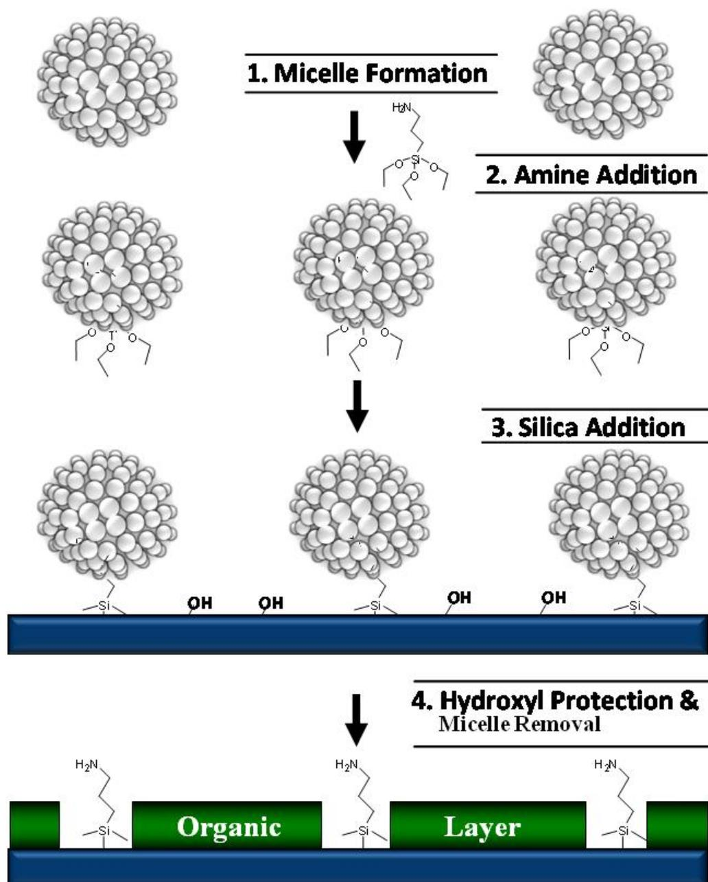
**Figure 1.4.** Micellar Templating Proposed Scheme. Micellar deposition of alkoxyaminosilane groups on silica for the creation of isolated amine site.
