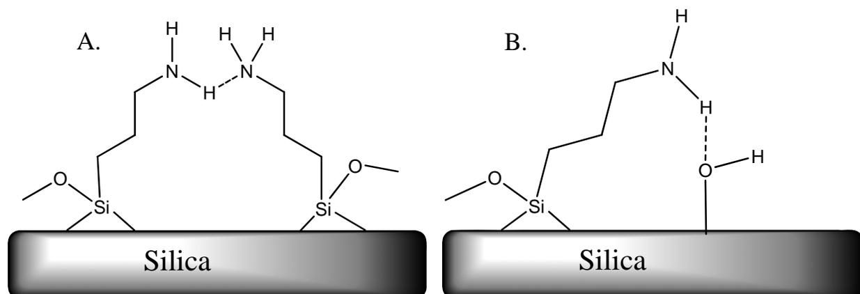
**Figure 1.2.** Amine Group Interactions. Amine groups are capable of interacting with (a) adjacent amine groups and (b) free hydroxyls on the surface of silica.
