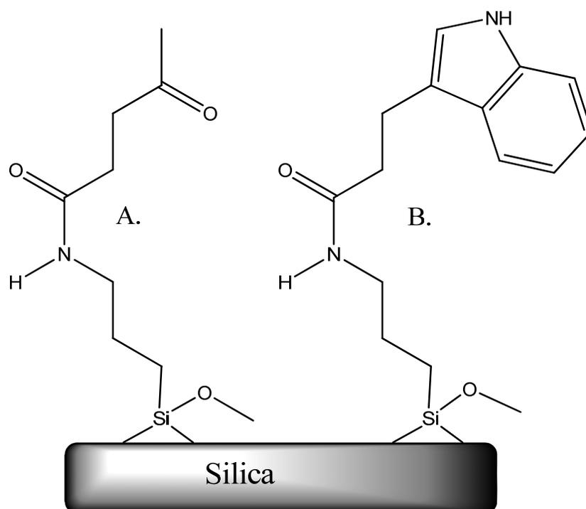
**Figure 1.6.** Silica Anchored Fluorophore and Fluorescence Quenching Molecules. Silica can be modified with various organic moieties such as (a) the fluorescence acceptor, levulinic acid, and (b) a fluorophore, indole propionic acid. Such modifications involve the synthetic coupling to the anchored amine sites on the silica surface.
