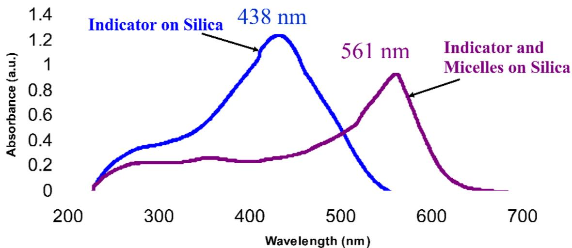
**Figure 3.3.** Reflectance UV-visible spectrum of silica wetness impregnated with an indicator, phenol red, (A) and with a solution of indicator stirred with micelles (B). A significant shift from 438 to 561 nm occurred with addition of micelles to the wetness impregnation solution containing phenol red.
