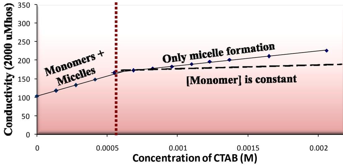
**Figure 3.2.** Determination of the Critical Micelle Concentration (CMC) Using Conductance Measurements. The conductivity of a 5mM TRIS buffer solution was monitored with increasing CTAB surfactant concentration. The CMC was determined as the concentration where the two linear regions of different slopes intersect.
