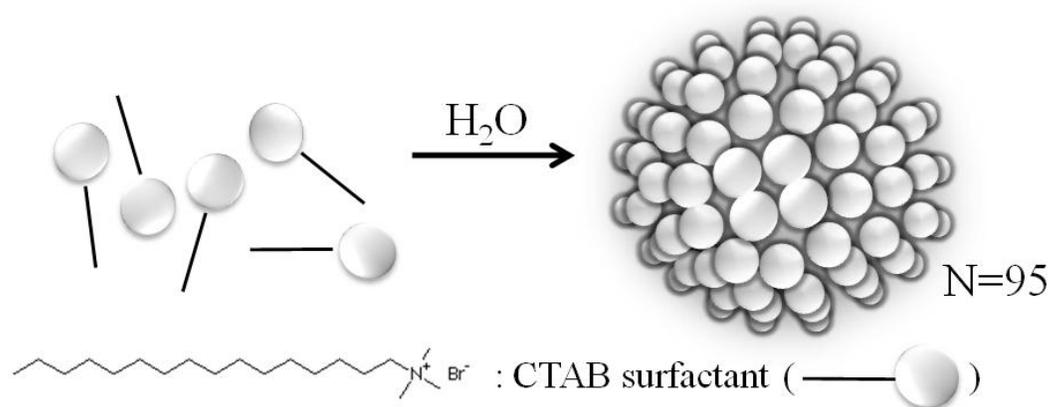
**Scheme 3.1.** Surfactant Monomer Aggregation Mechanism for CTAB Micelle Formation in Aqueous Environments. This scheme shows the assembly of 95 CTAB surfactant monomers to form one micelle template.
