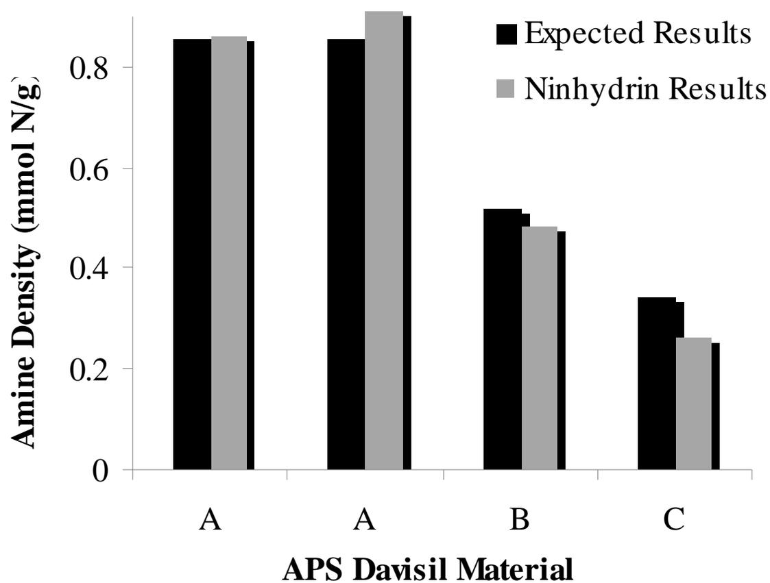
**Figure 2.3.** Ninhydrin Tests on Grafted APS Silica Materials. The two samples with 0.857 mmol/g loadings (Sample A) were tested by using different solutions on different days to test reproducibility from day-to-day. All expected loadings and experimental results can be found in Table 2.2.
