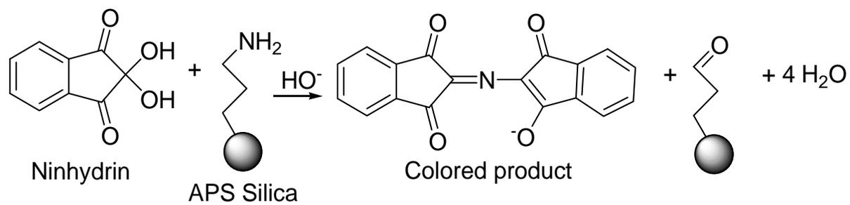
**Figure 1.5.** Ninhydrin Reaction with Aminopropyltriethoxysilane (APS) Functionalized Silica
