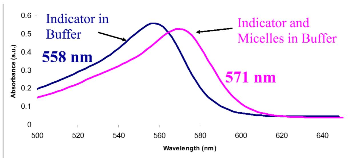
**Figure 3.4.** UV-visible spectrum of a 5mM TRIS buffer solution with Phenol Red in the absence (A) and in the presence of micelles (B).
