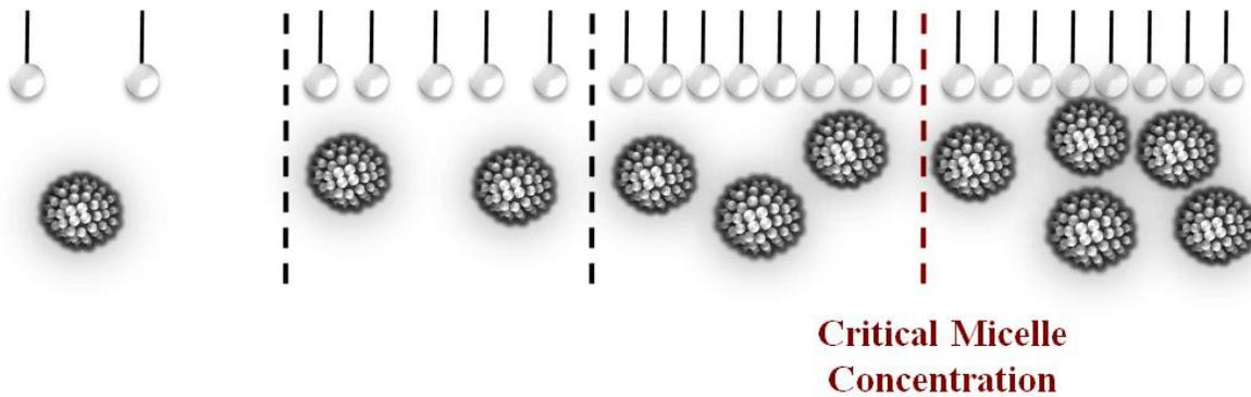
**Scheme 3.2.** Depiction of the Critical Micelle Concentration (CMC). This mechanism indicates that an increase in surfactant concentration initially increases the concentration of both the surfactant monomers and micelles in solution (Steps 1-3); however, the monomer concentration will become constant (Step 4) after the CMC and any surfactant addition contributes to micelle formation in solution.
