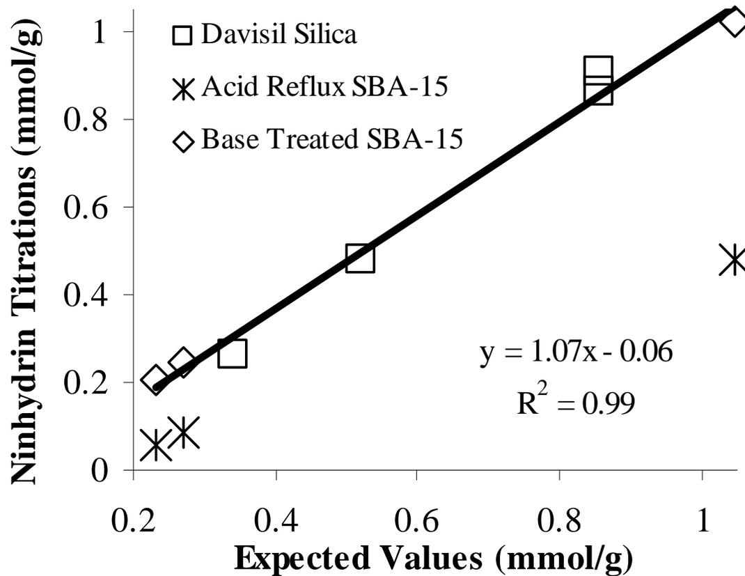
**Figure 2.5.** Parity Plot for Ninhydrin Titrations. Measured amine densities are plotted against the expected values.
