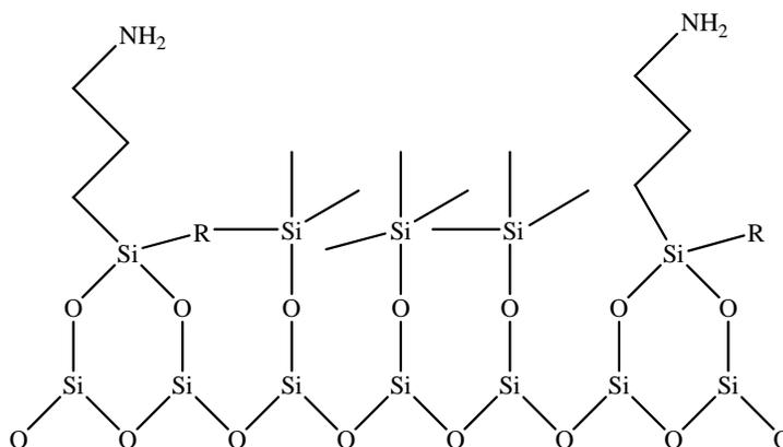
**Figure 1.3.** Aminoalkyl-Modified Silica. Isolated aminopropyltriethoxysilane grafted onto silica with subsequent protection of surface hydroxyls with tetramethyldisilazane.
