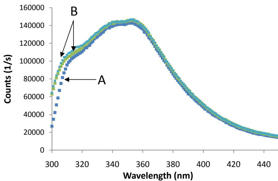
**Figure 4.3.** Fluorescence spectra of 100% donor covered APS grafted silica material (0.514 mmol/g) before (A) and after (B) the addition of excess activated acceptor (levulinic acid).
