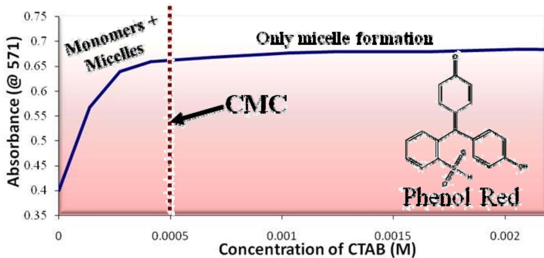
**Figure 3.1.** Determination of the Critical Micelle Concentration (CMC) Using UV-visible Spectroscopy. The absorbance (571 nm) of a 5mM TRIS buffer solution containing phenol red was monitored with increasing CTAB surfactant concentration. The CMC was determined as the concentration at which point the absorbance is no longer affected significantly by CTAB surfactant additions. The structure of the phenol red indicator is shown on the graph.
