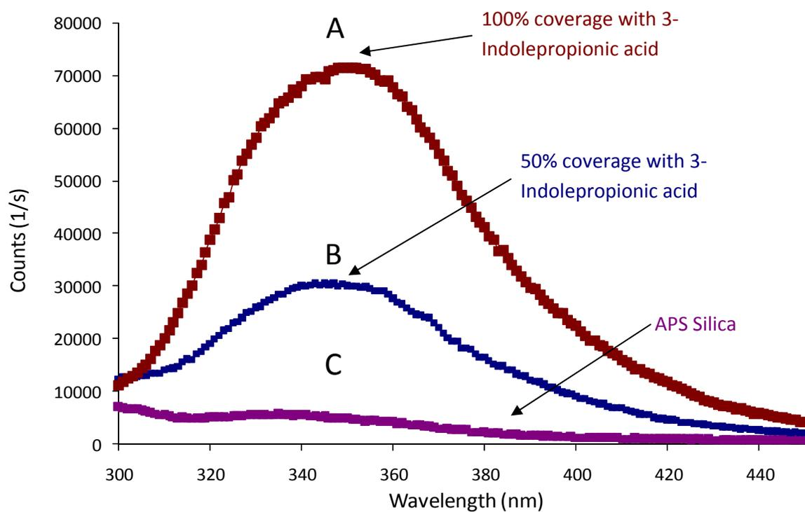
**Figure 4.2.** Fluorescence spectra of APS modified grafted Davisil silica of 0.857 mmol APS/g loading when 100% (A), 50% (B), and 0% (C) of the amine sites are reacted with the fluorescent donor, 3-Indolepropionic acid.
