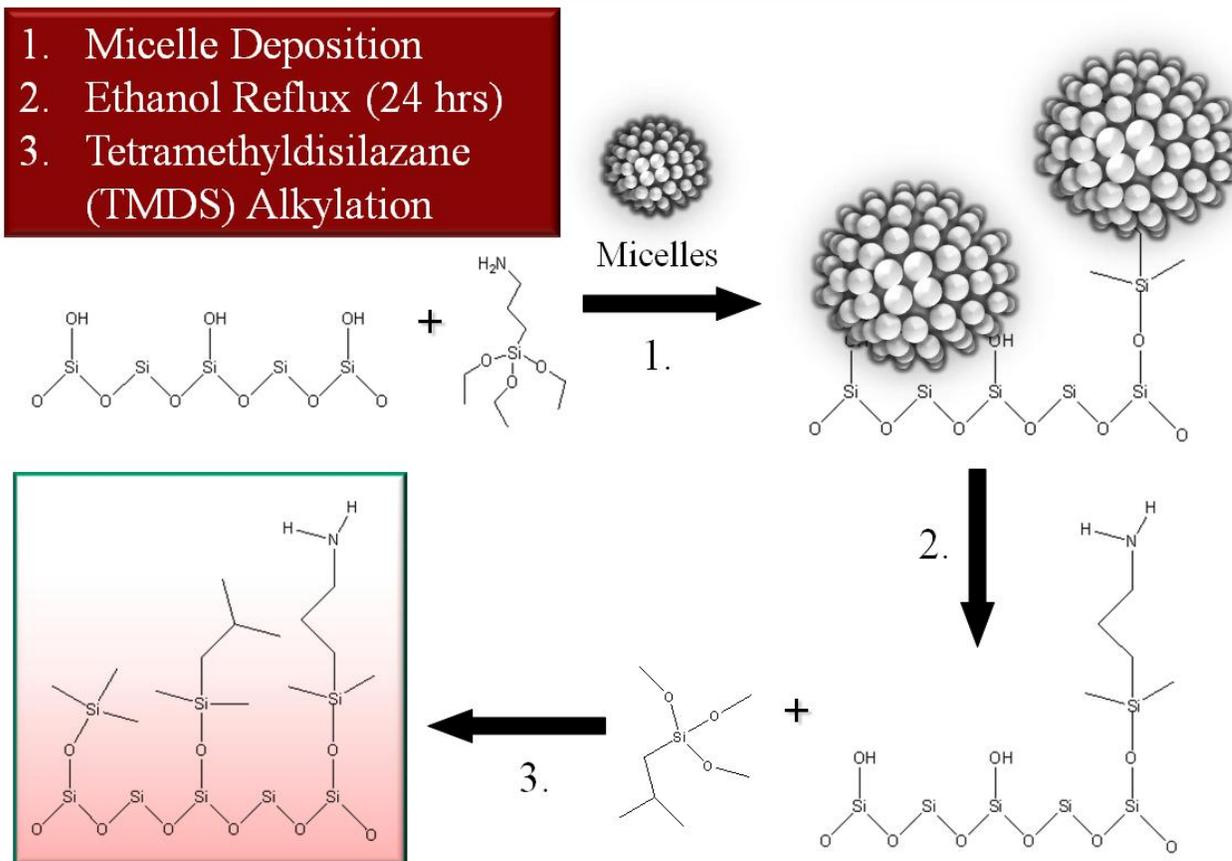
**Scheme 3.3.** Micelle Templating and Free Hydroxyl Alkylation for Elimination of Amine-Amine and Amine-Surface Interactions. The scheme proposed to create isolated sites involves silane encapsulation, micelle adsorption on Davisil silica, micelle removal, and surface alkylation with various alkylating reagents. Specifically, the APS deposition, micelle removal, and surface alkylation have all been verified using IR spectroscopy, and all spectra are provided in the Appendices B-C.
