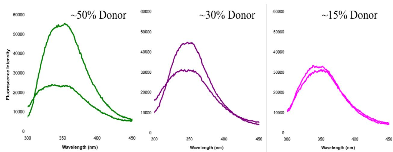
**Figure 4.4.** Quenching of different anchored 3-Indolepropionic acid loadings on APS silica materials by an acceptor, levulinic acid. The fluorescence intensities of three APS grafted silica materials with donor coverages of 50%, 30%, and 15% were monitored before and after the anchoring of levulinic acid. For all samples, the peak of lesser intensity represents the trial after acceptor addition.
