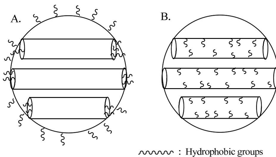
**Figure 1.1.** Various methods for silica functionalization include (a) post-synthetic modifications and (b) one-step co-condensation techniques (28).
