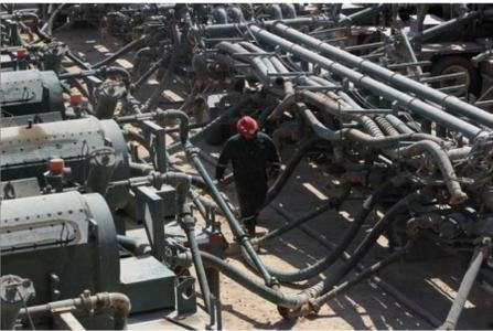
An oil worker walks past the manifold (right) and frac pumps (left) at a Chesapeake Energy hydraulic fracturing operation near Carrizo Springs. Hydraulic fracturing is a method of removing oil and gas from rock formations such as the Eagle Ford shale formation. Photo: JOHN DAVENPORT/SAN ANTONIO EXPRESS-NEWS
