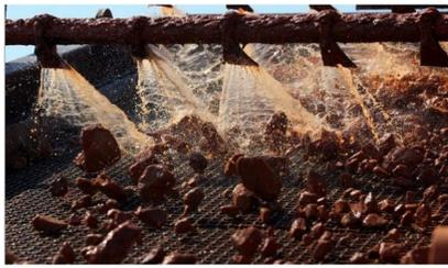
Sand and stone mined near Brady is washed and sent through a vibration and screening process. Much of the sand produced there is used by the oil and gas drilling industry in areas such as the Eagle Ford shale formation. Photo: JOHN DAVENPORT/SAN ANTONIO EXPRESS-NEWS
