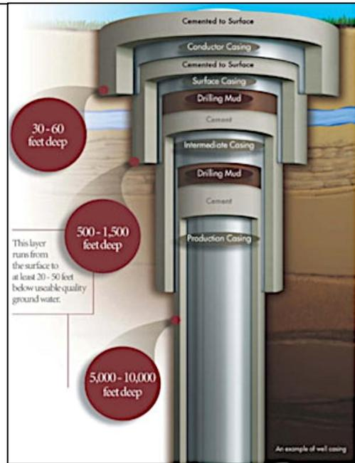
**Figure 2—Design of the well casings used to protect aquifers**
