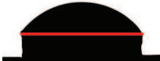
Figure 3: Image of a 3MP drop of radius 1 mm acquired at the beginning of the experiment. The red horizontal line indicates the surface of the platform. The contact angle is approximately 50^\circ .
