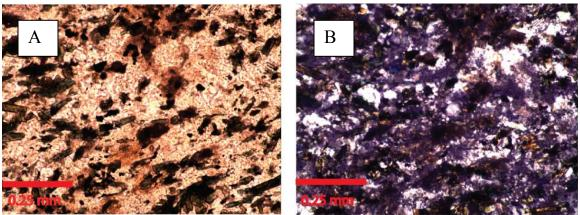
**Figure 8.** Photomicrographs (20X) of sandstome sampe PCC-11 (A = uncrossed polars; B = crossed polars). Notice textural and compositional immaturity (angular grains, high clay content) that help designate a proximal source.
