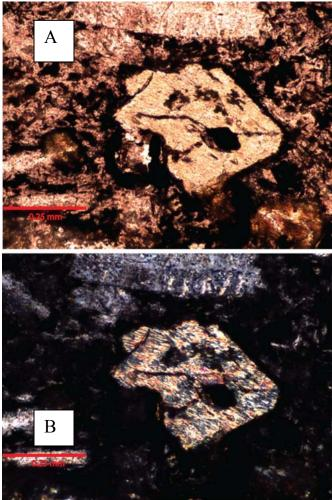
**Figure 9.** Photomicrographs (20X) of sample PCC-08 (A = uncrossed polars; B = crossed polars) showing distinct cleavage of an amphibole grain with replacement through hydrothermal alteration.
