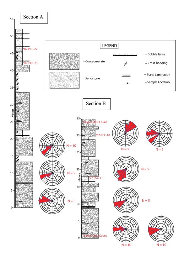
**Figure 4.** Stratigraphic Column with corresponding paleoflow from imbrication readings. The two sections are separated by a ravine in outcrop, but there is no evidence for fault displacement.
