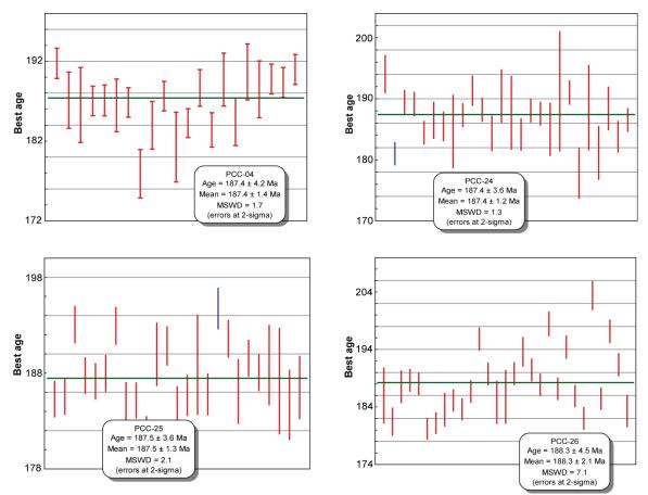
**Figure 13.** Best fit ages for zircon from four individual cobble clasts. Length of red lines accounts for potential error of each zircon crystal while green line highlights best age without factoring in error. X-axis is individual zircon grains from each cobble sample.
