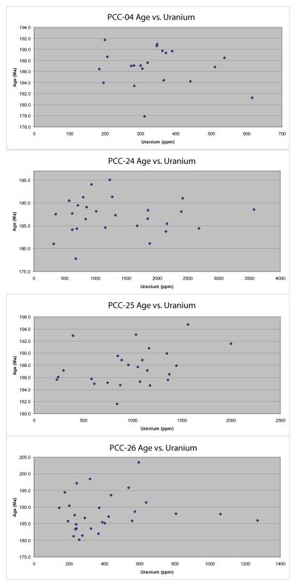
**Figure 14.** Igneous cobble ages plotted against uranium concentration show no linear trends that would indicate damaged or contaminated zircon grains.
