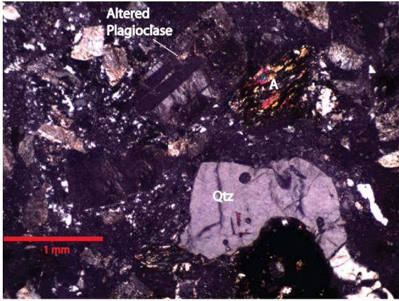
**Figure 10.** Photomicrographs (5X) of sample PCC-12 under crossed polars showing an amphibole grain (A) along with embayed quartz (Qtz), which is characteristic of quartz in volcanic rocks. Amphibole is key in classifying igneous rocks because it is usually found in intermediate to felsic rocks, and is not a product of hydrothermal alteration.
