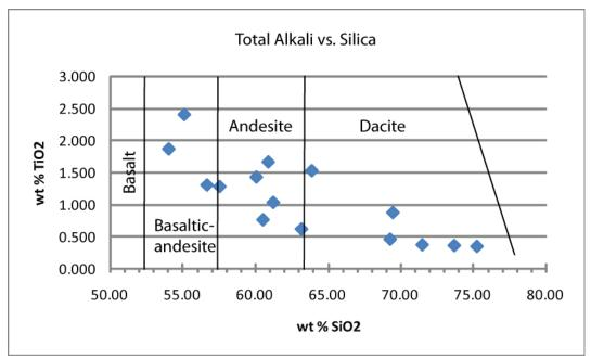
**Figure 15.** Major element geochemistry ploting total alkali vs. silica. Chemical classification and nomenclature for volcanic rocks by Le Maitre et al. (1989). Data indicate a largely Andesite-Dacite composition for the source of the PCC.
