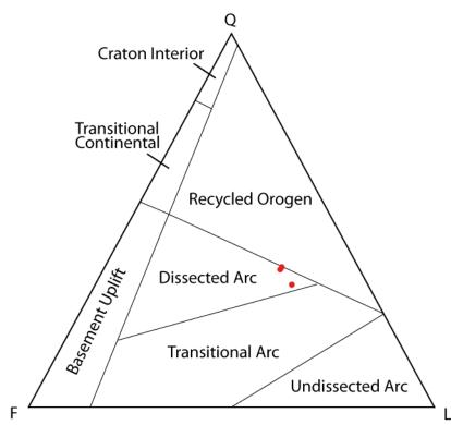
**Figure 7.** QFL diagram with provenance fields from Dickinson (1993). Point count data (red dots) suggest a dissected arc source for the PCC.
