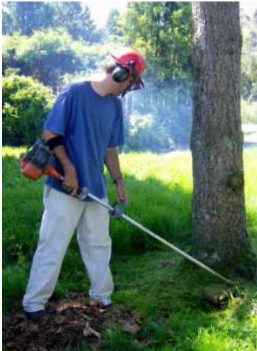
Fig. 1 A typical string trimmer is supported by a grip adjacent to the engine (left) and a loop-shaped handle (right) located further down the shaft [4]
