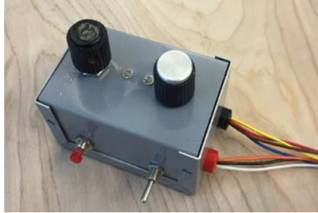
Figure 2. Control Box. Left knob controls motor sweep, right knob controls strobe time, button allows color selection, three position switch allows mode selection
