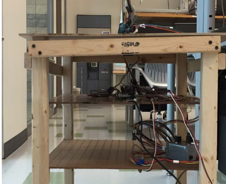
Figure 15. Implemented wiring. All connections are soldered, all wires are zip tied down, all wires going to the same location are taped together
