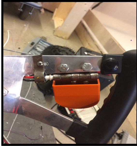
Figure 7: Throttle potentiometer assembly with throttle cover
