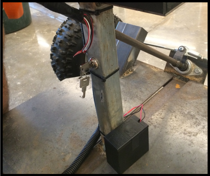
Figure 3: Key-lock power switch and battery housing
