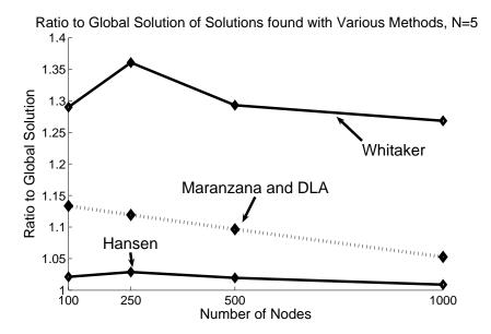
Figure 3: The average objective value as a ratio of the global solution versus |V| with N = 5. Each technique appears to improve its solution quality as |V| increases.
