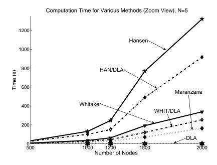
Figure 4: The computation time for the heuristics plotted versus |V|.
