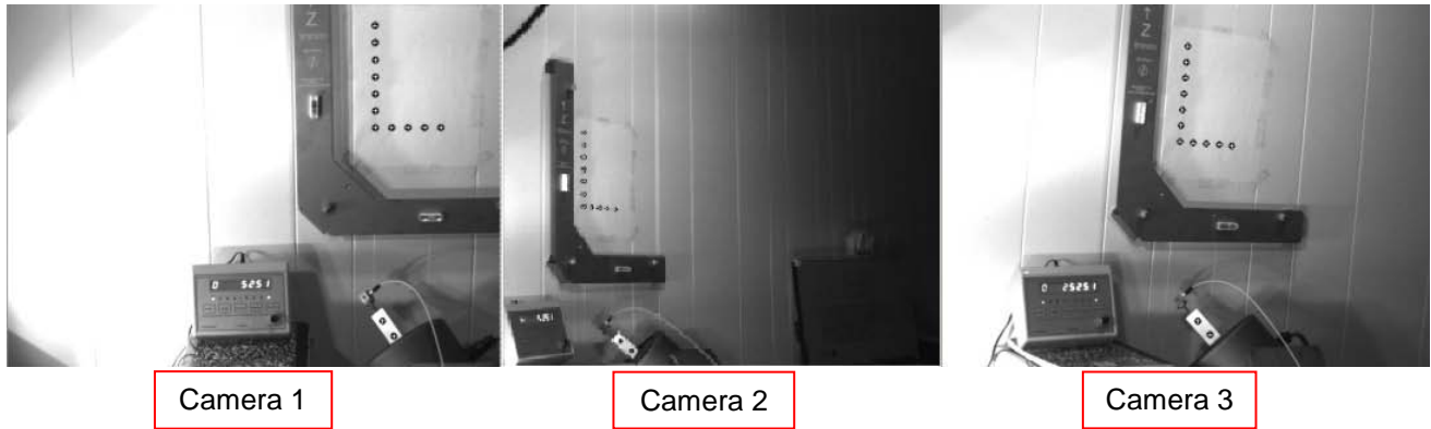
Fig. 6: Experimental images used to calculate off-axis acceleration of a sinusoidally-driven shaker. In this experiment, the shaker was rotated by 30 degrees with respect to both the x- and z-axes defined for the space. Both the lighting schemes and camera positions were slightly different than those chosen for the on-axis shaker experiment.
