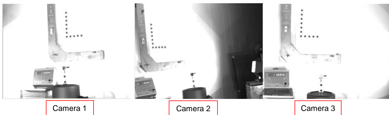
Fig. 5: Once set of the experimental images (epoch) used to calculate acceleration of a sinusoidally-driven shaker. In this experiment, the oscillating shaft was aligned with the horizontal (y) axis of the pictured coordinate axes.
