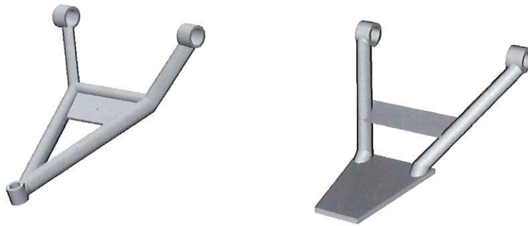
Figure 2.3: View of Front and Rear Control Arms
