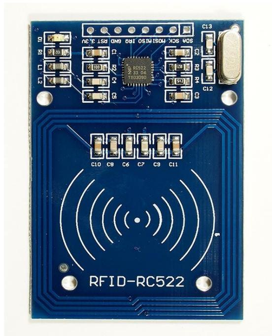
Figure 9. MFRC-522 RFID Reader
