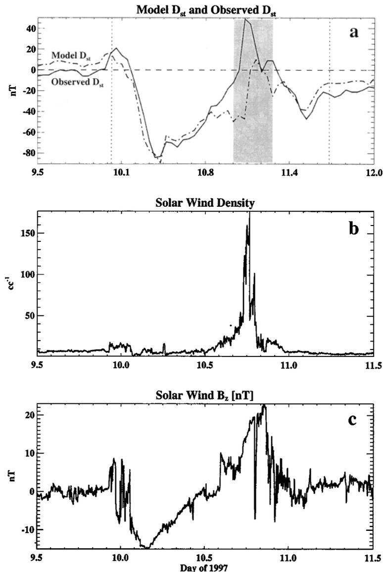
**Figure 2.** (a) Modeled and observed  $Dst$  (not pressure-corrected) for January 9–12, 1997; (b,c) solar wind conditions. The shaded region is during a solar wind pressure pulse which is out of range for the model.
