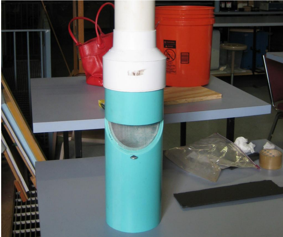
Figure 14. Primary filter after construction
