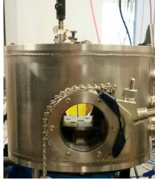
Figure 3. Photo of the pressure chamber in which the P/G experiments were conducted. The drop evaporation rate was measured using the shadowgraph technique through the side windows.
