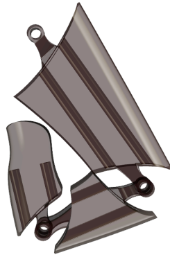
Figure A3. Contracted finger - bottom wire pulled
