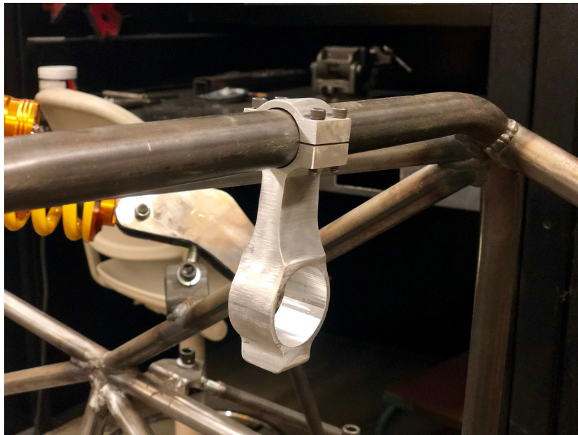
Figure 8. CNC manufactured steering column support fixed to the vehicle chassis
