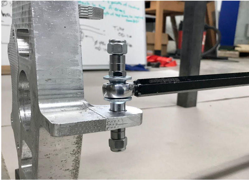
Figure 11. Steering end links making the tie rod connection to the uprights. The tie rod end links are connected to the upright at an angle with the horizontal plane of less than 5 degrees.
