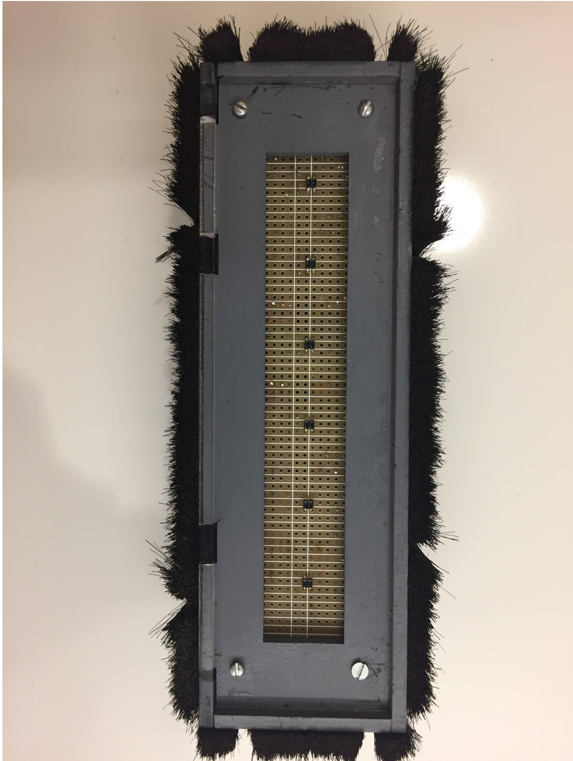
Fig. B1.3 IR Array as seen from bottom showing IR LED/sensor packages.
