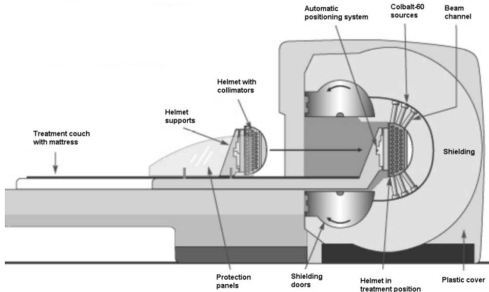
Figure 1: Gamma Knife cut away.<sup>1</sup>
