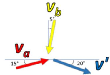
Figure 2: Skid mark angles for car crash
