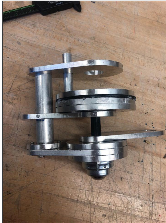
Figure 6. Assembled brake with the 3D printed shaft
