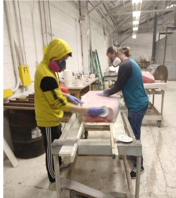
**Figure 6.** Sanding of top body panel mold after a fiberglass application
