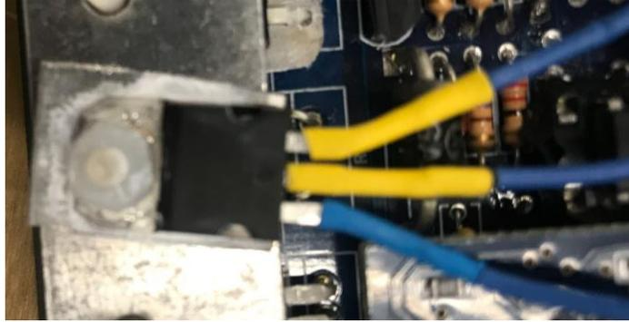
**Figure 25.** BIP373 Transistor modification for dual spark configuration
