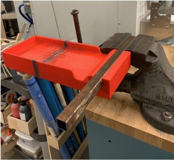
**Figure 16.** The 3-D printed headrest is composed of three parts with the interface being secured using aircraft grade epoxy
