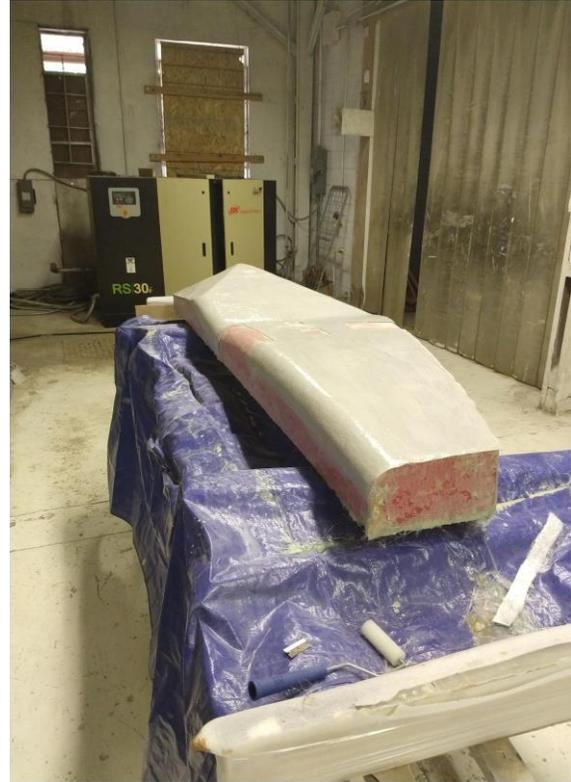
**Figure 8.** The finished right-side panel, cut, primed, and ready to be put on the car
