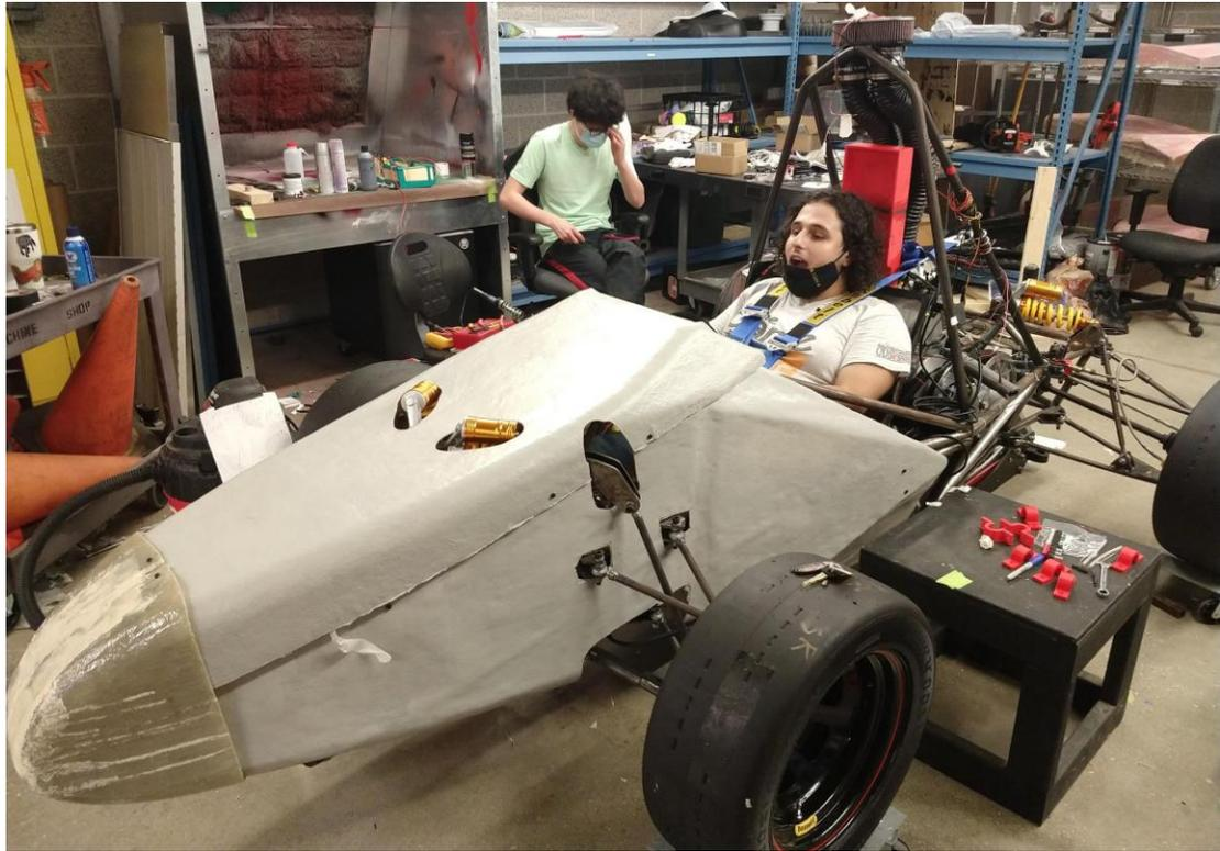
**Figure 9.** Completed body panels attached to the car chassis
