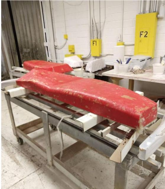
**Figure 5.** Right side body panel mold with initial fiberglass layer
