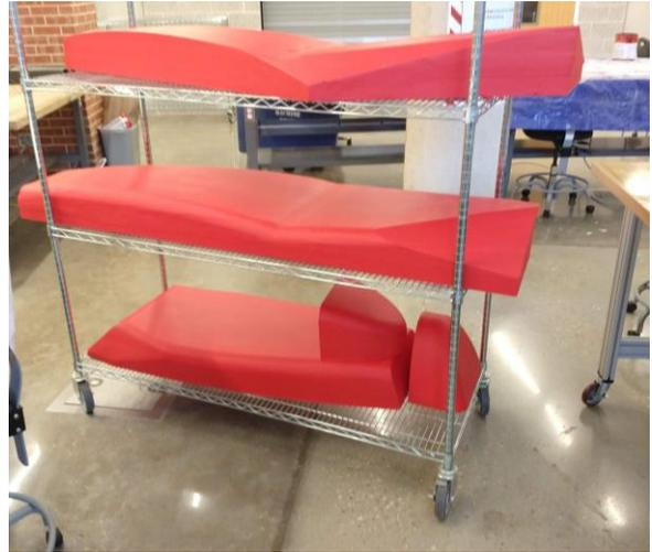
**Figure 4.** The molds after being assembled, sanded, painted, and ready to be fiberglassed
