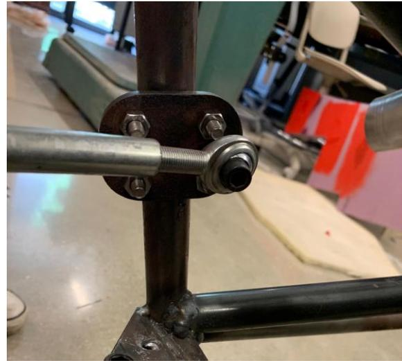
**Figure 19.** Alignment mounting point
