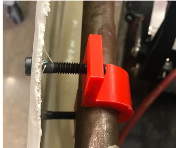
**Figure 11.** 3-D printed body panel mounts securing body panels to chassis
