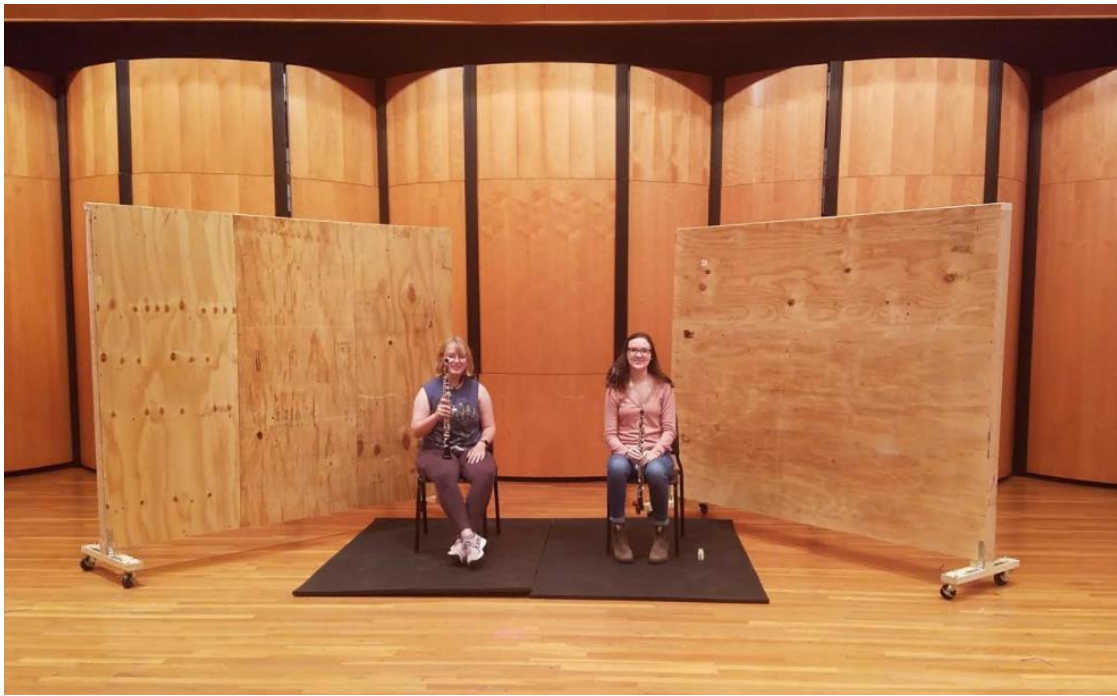
Figure 13. Visual aid for combination of Absorptive Mat and Reflective Walls, used in woodwind testing (oboe).
