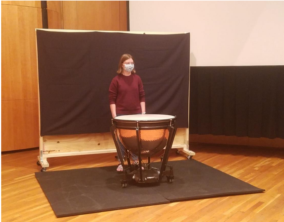
Figure 12. Visual aid for combination of Absorptive Mat and curtain attached to the back of a Reflective Wall, used in percussion testing (timpani).
