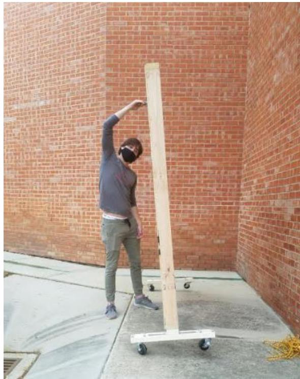
Figure 20. Tipping tests for the Reflective Wall components.
