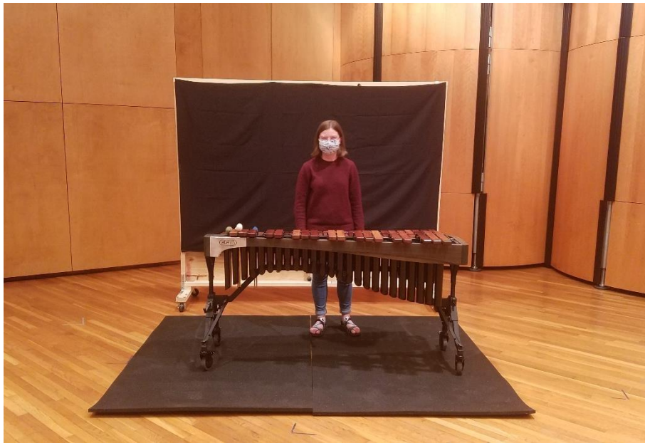
Figure 14. Visual aid for combination of Absorptive Mat and curtain attached to the back of a Reflective Wall, used in percussion testing (marimba).
