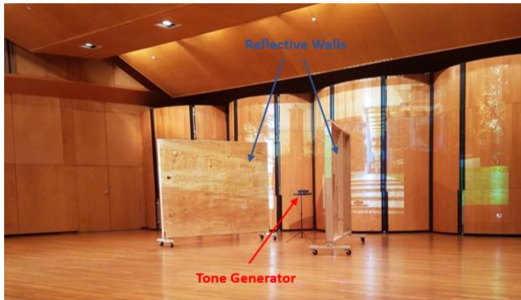
Figure 5. Experimental set-up for Test 3 of the Reflective Walls. The tone generator and its stand are placed between the two walls, which flank the generator at a sharp angle.
