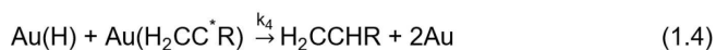
Scheme 1. Mechanism for 1-octyne hydrogenation based on the literature; HCCR is 1-octyne and H 2 CC* R is partially-hydrogenated 1-octyne.
