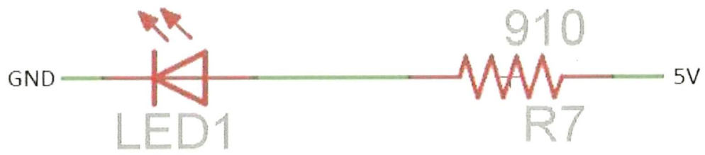
Figure A6: Doll Emitter Circuit
