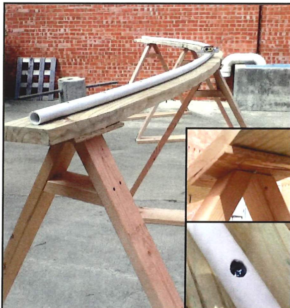
Figure 5: a. The PVC laser track with wood support structure. b. bases are not permanently attached to the track to allow for dismantling and storage. c. bolts are placed through holes in the top of the PVC to allow the sled to slide without catching.
