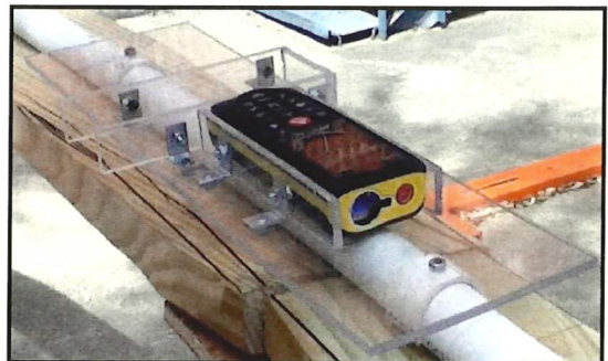
Figure 6: Plexiglas sled has slots to hold the Leica D8 during measurement and calibration. Cut PVC sections allow the sled to slide while still providing enough friction to keep the sled from tipping.
