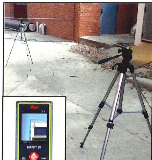
Figure 1: a. Laser distance measurement in a normal setup. The Leica D8 is placed on a tripod held stationary and aimed at a stationary target. b. The 4x zoom camera included in the Leica D8 model.
