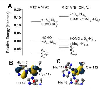
**Figure 7.** Frontier molecular orbitals. (A) Relative  $\beta$ -spin frontier molecular orbital diagram of M121A Ni<sup>II</sup>Az and M121A Ni<sup>II</sup>-CH<sub>3</sub> Az obtained from B3LYP/def2-TZVP calculations. (B) Contour plot of the  $\beta$ -d<sub>xz</sub> orbital from M121A Ni<sup>II</sup>-CH<sub>3</sub> Az. (C) Contour plot of the  $\beta$ -d<sub>yz</sub> orbital from M121A Ni<sup>II</sup>-CH<sub>3</sub> Az.
