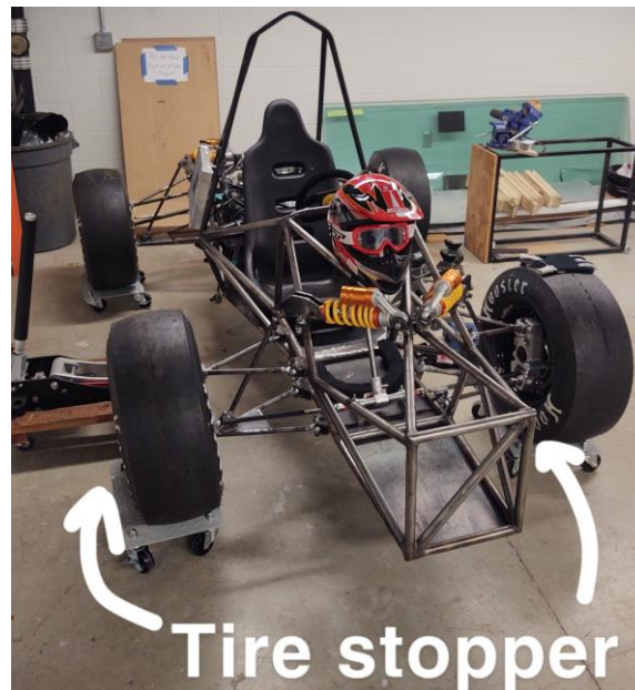
Figure 3.4.2. Place something on this side of the front tires so as to restrict any movement of the tires.
