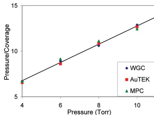
**Figure 8.** Higher-pressure adsorption data plotted in a linear form of the Langmuir equation. The line is a fit to all the data and has been used to convert the integrated infrared peak areas to coverage according to eq 1 (see text).
