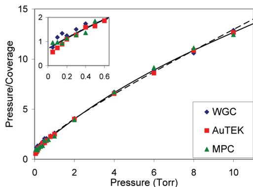
**Figure 6.** Room-temperature adsorption data for the three Au nanoparticle catalysts plotted over the entire pressure range in a linear form of the Langmuir equation. The data show a slight deviation from ideal Langmuir behavior over the large pressure range. A smooth, polynomial curve fit (solid line) has, therefore, been used to determine the binding constant as a function of coverage. Alternatively, the dashed line is a two-site model fit (see text).
