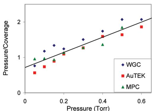
**Figure 7.** Lower-pressure adsorption data plotted in a linear form of the Langmuir equation. Within experimental reproducibility, the three catalysts have similar coverage dependence. The line is a fit of all data over this pressure range, demonstrating near-ideal Langmuir behavior.
