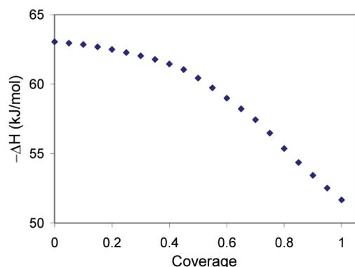
**Figure 10.** Enthalpy for CO adsorption on the three Au catalysts as a function of coverage. These values were determined from the binding constants at room temperature (see Figure 9) and a literature value for the entropy contribution,  $T\Delta S = -44$  kJ/mol (see text).
