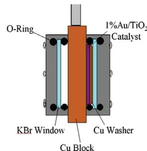
**Figure 1.** Cross section of the sample cell for infrared transmission spectroscopy of gold-supported catalysts. The Au/TiO<sub>2</sub> catalyst is pressed into a 30 × 30 Ti mesh and mounted inside the copper cell.
