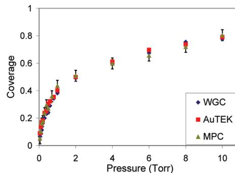
**Figure 5.** Langmuir isotherm plot for the three Au nanoparticle catalysts at room temperature. Coverage was determined from a Langmuir fit of the data at higher pressures (see text and Figure 8). Each point is the average of two to five individual experiments. Error bars representing one standard deviation are included for the MPC data. Within experimental reproducibility, all three catalysts exhibit similar coverage dependence.
