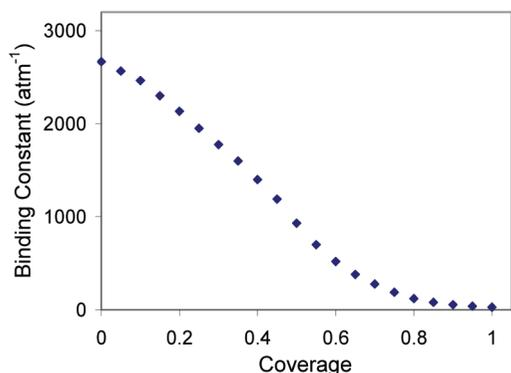
**Figure 9.** Binding constant for CO adsorption on Au nanoparticle catalysts at room temperature. The binding constant was determined according to eq 1 and the smooth curve in Figure 6. This analysis yields values of  $\Delta G$  for CO adsorption that varies from  $-20$  to  $-8$  kJ/mol for low to high coverage, respectively. Since data were not collected for coverages above 0.8, the binding constants above 0.8 are an extrapolation of the fit.
