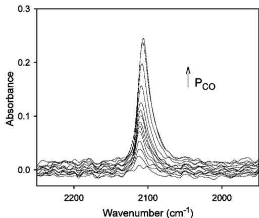
**Figure 2.** Infrared transmission spectra of CO adsorbed on the Au nanoparticle catalyst at room temperature (1% Au on TiO<sub>2</sub>, WGC catalyst, 34 mg pellet). CO pressure was increased from 0 to 10 Torr. Integrated peak area represents the CO coverage at each pressure. The CO peak shows a red shift with increasing coverage.
