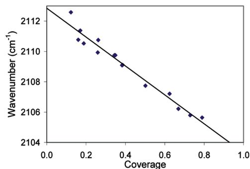
**Figure 4.** Infrared CO peak position showing a red shift with coverage. Coverage was determined from a Langmuir fit of the integrated peak area at higher CO pressures (see text and Figure 8). The line is a fit to the data, showing an approximately linear relationship.
