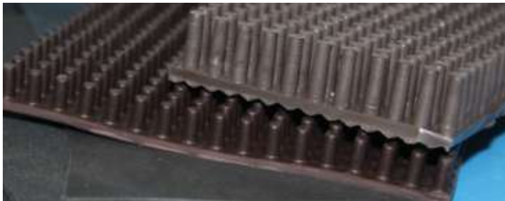
Fig. 3 Studded rubber mats used as wraps in the attenuation tests. The studs on the bottom mat were 0.25 in long, the studs the top mat were 0.50 inch long.
