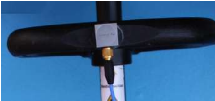
Fig. 4a Accelerometer mounted on handle, aligned with a basicentric coordinate system. Note the flat milled into the surface of the handle facilitates a secure coupling
