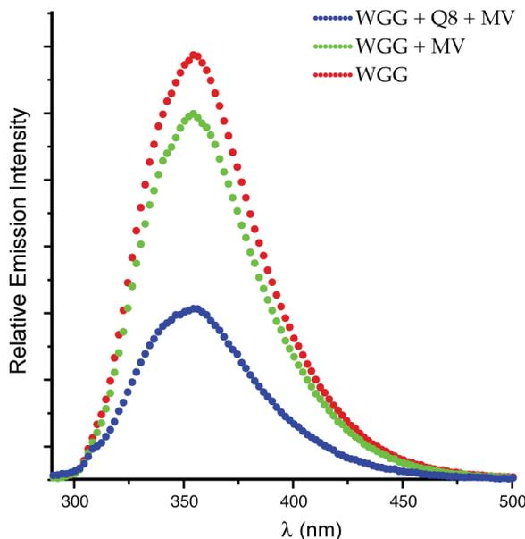
**Figure 6.** Fluorescence emission spectra for WGG unbound (red) and in the presence of one equivalent of MV (purple) or Q8•MV (blue). All spectra were obtained with excitation at 279 nm at 25 °C at a concentration of 12.5  $\mu$ M in 10 mM sodium phosphate, pH 7.0. Significant quenching of indole fluorescence is apparent in the
