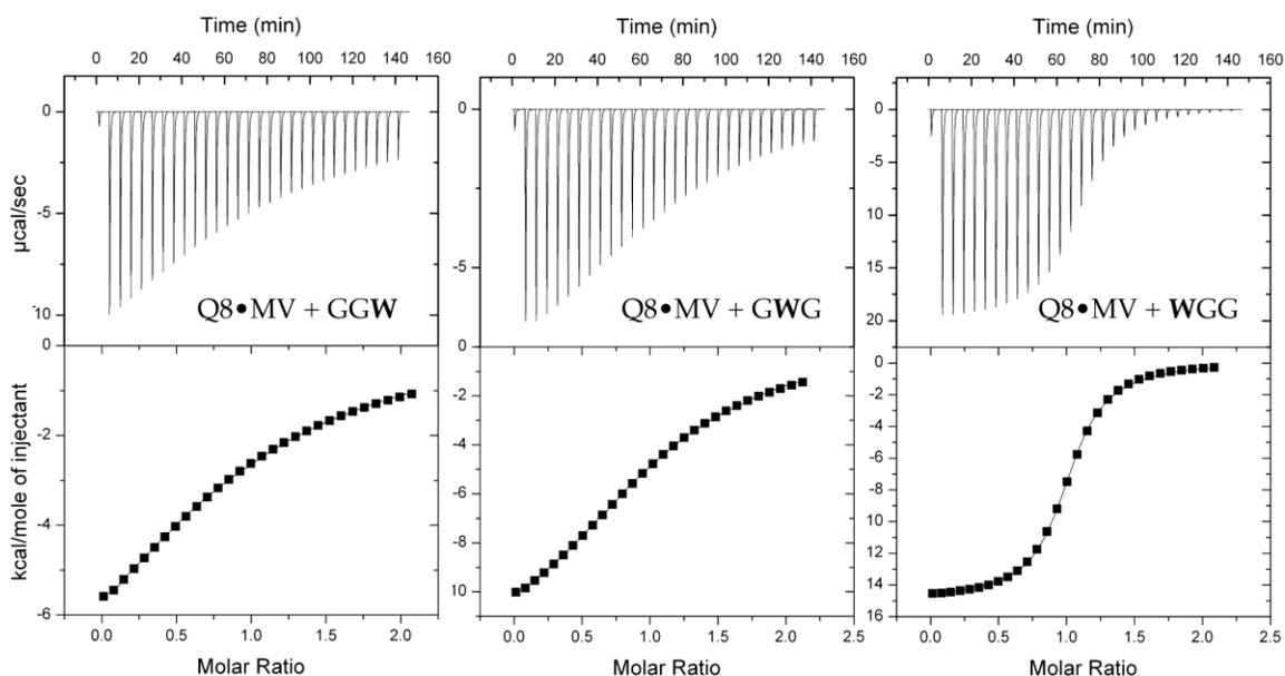
**Figure 4.** ITC data for the complexation of Q8•MV with GGW (left), GWG (center), and WGG (right) at 27 °C in 10 mM sodium phosphate buffer, pH 7.0. WGG and GGW were titrated at 5 mM into a 0.5 mM solution of Q8•MV. GWG was titrated at 2 mM into a 0.2 mM solution of Q8•MV. The top plot shows the raw data for power applied as a function of time. The integrated enthalpy values are plotted at bottom as a function of the molar ratio of
