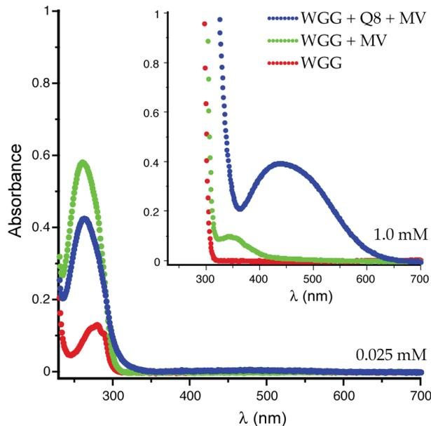
**Figure 5.** UV-visible spectra of WGG unbound (red) and in the presence of one equivalent of MV (purple) or Q8•MV (blue) at 25 °C in 10 mM sodium phosphate, pH 7.0. Data were obtained at concentrations of 0.025 mM and 1.0 mM (inset) in order to display all relevant peaks within the linear dynamic range of the spectrophotometer. At 1.0 mM, new charge-transfer bands are apparent at 350 nm for WGG + MV
